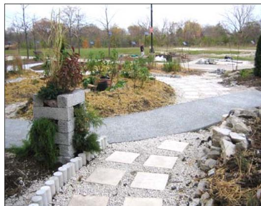
sites in general. Using pervious concrete pathways, recycled concrete aggregate, pervious rip-rap, and an extensive network of storm swales and biofiltration checkpoints, the garden has become an engineered “living” entity performing ecosystemic services rendered innocuous by previous development. In this sense, it is both a re-creation, and man-made improvement upon, natural processes which would otherwise handle the issues mentioned.
